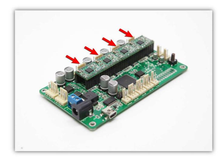
These drivers control the current that flows through each motor. To do that correctly each of them needs to be calibrated. Take your multimeter and a ceramic screwdriver (a normal screwdriver will also work but be very careful not to touch anything else but the trimmer on the driver boards as you can cause a short circuit).
