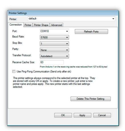
Change the settings on this tab to the ones below (for the "Port" setting you should use the Virtual COM Port on which your computer is communicating with the K8200. See the section about driver installation at the beginning of this chapter for more information.)
