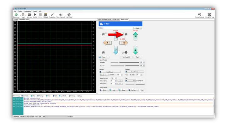
As soon as you have pressed this button the print bed will move towards the micro switch that your finger is resting on. Quickly press the micro switch. If the micro switch is working correctly the bed will stop.
