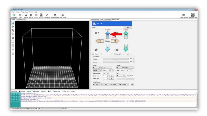
The Y AXIS should go **FORWARD** 10 mm, everything should go smoothly. If the Y AXIS does not move or moves in the opposite direction you wired something wrong. Find and correct the fault before continuing.
