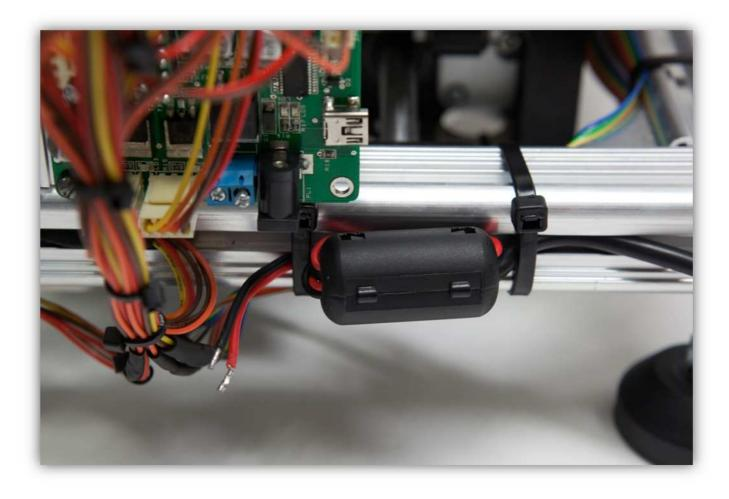
Connect the wires to the blue screw connector. **Notice the polarity. The red wire is positive and the black is negative.**
