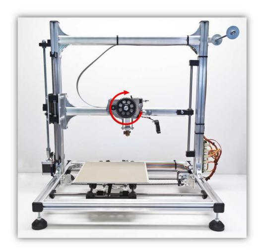
The extruder motor should turn smoothly. If the LARGE GEAR does not move or moves in the opposite direction you wired something wrong. Find and correct the fault before continuing.
