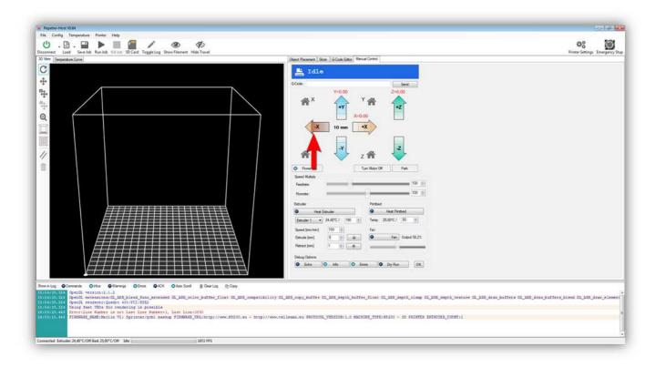
The X AXIS should go **RIGHT** 10 mm, everything should go smoothly. If the X AXIS does not move or moves in the opposite direction you wired something wrong. Find and correct the fault before continuing.
