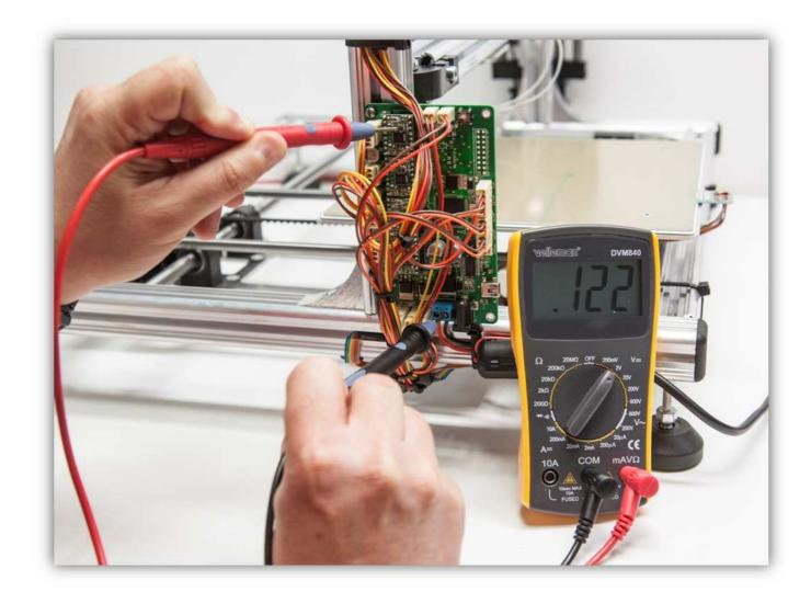
Adjust the little trimmer on the driver with the ceramic screwdriver until you measure **0.425V.**
