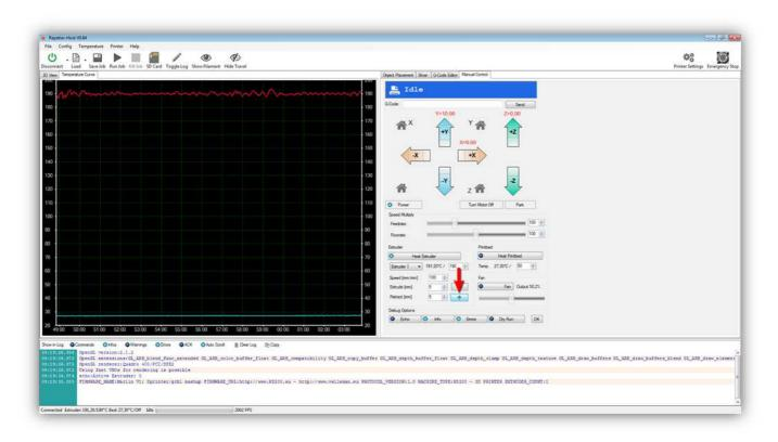
The extruder motor should turn a bit and make the large gear turn to the LEFT.
