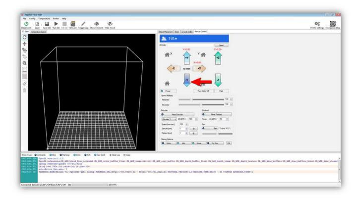
The Y AXIS should go **BACK** 10 mm, everything should go smoothly. If the Y AXIS does not move or moves in the opposite direction you wired something wrong. Find and correct the fault before continuing.
