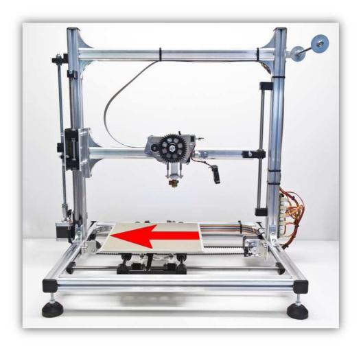
Put your finger on the micro switch of the X AXIS, do not press it.
