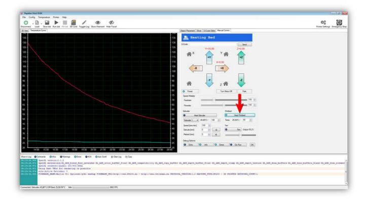
The BLUE line in the temperature graph should start to rise, and you should see the current temperature of the HEATED BED PCB rise.
