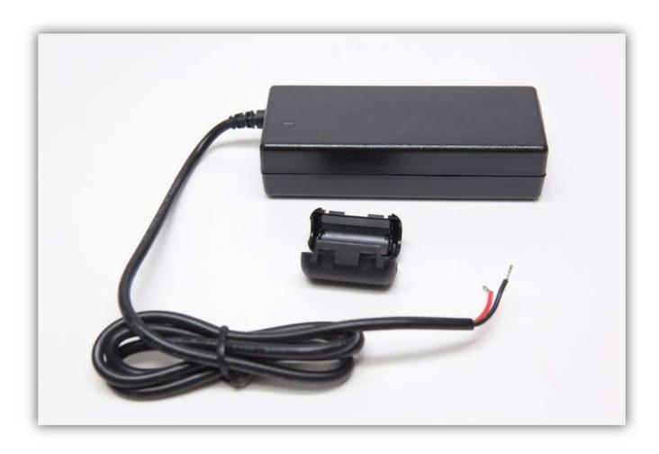
First strip the end of the cable so you have 15 cm (5.9") of free wire. **Be careful not to cut too deep while you are stripping the cable.**
