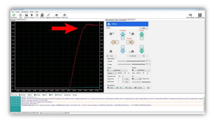
While the extruder is hot we can test the extruder motor. For safety reasons, the motor cannot turn when the extruder is cold. First check the values in the following boxes.
