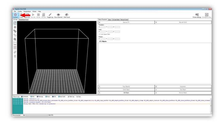
The text on the button should change from "Connect" to "Disconnect".
