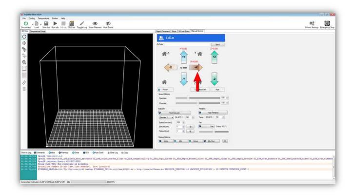
The X AXIS should go **LEFT** 10 mm, everything should go smoothly. If the X AXIS does not move or moves in the opposite direction you wired something wrong. Find and correct the fault before continuing.
