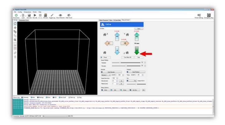
The Z AXIS should go **DOWN** 10 mm, everything should go smoothly. If the Z AXIS does not move or moves in the opposite direction you wired something wrong. Find and correct the fault before continuing.
