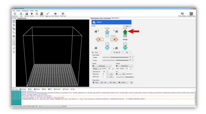
The Z AXIS should go **UP** 10 mm, everything should go smoothly. If the Z AXIS does not move or moves in the opposite direction you wired something wrong. Find and correct the fault before continuing.
