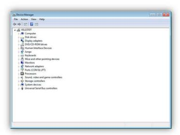
Under "Ports (COM&LPT)" you should find an entry with the name: USB Serial Port and a COM Port number between brackets. (The number you see on your computer can be totally different from the one you see here.) Remember this number as you will need it later.
