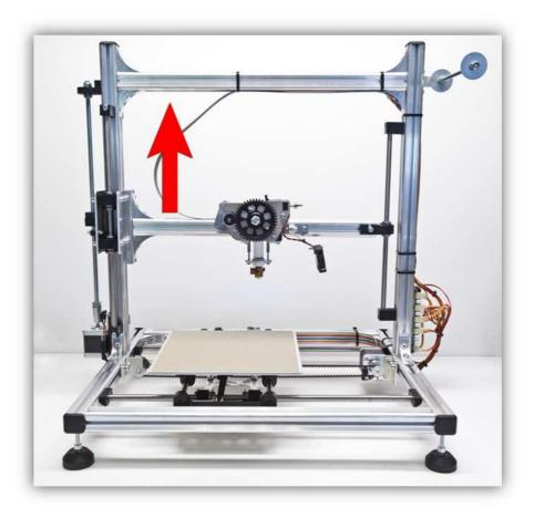
Put your finger on the micro switch of the Z AXIS, do not press it.
